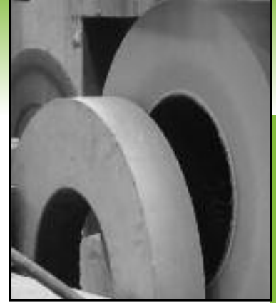
RIGHT: Goodson's slicing machine can remove as little as .015" from your wheel.
