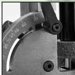
ABOVE: Easy to read scale is marked in 1° increments
