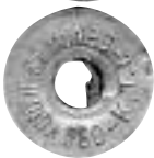
melted center reveals overheating
