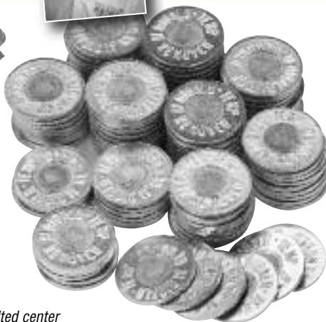
melted center reveals overheating
